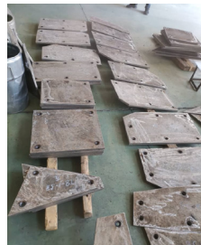
Pump Box Liner
