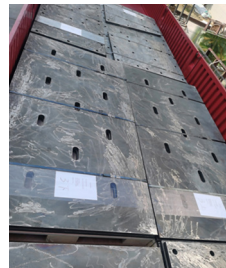
Pump Box Liner
